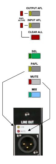
**PAFL key** Selects either the PFL (pre-fade listen) or AFL (after-fade listen) signal to the engineer's headphones / local monitor depending on the setting of the AFL keys below the PAFL meters. Press PAFL keys to toggle them on or off, or use the CLEAR ALL key in the master section to turn off the current selection. The associated yellow CHK indicators light on the iDR10 MixRack and iLive Surface audio modules while PAFL is active. The T Series does not provide these indicators.
